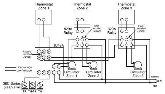
Figure 8. 8J48A - 24 Volt Systems Zoned with Circulators
